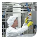
Cleaning in Place (CIP) systems automate the cleaning cycle, ensuring repeatable results. It is important to understand how the system works in order to ensure the correct program is utilised and resources are not wasted.
